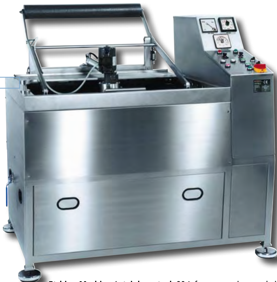
Etching Machine / stainless steel, 90 L for magnesium and zinc
